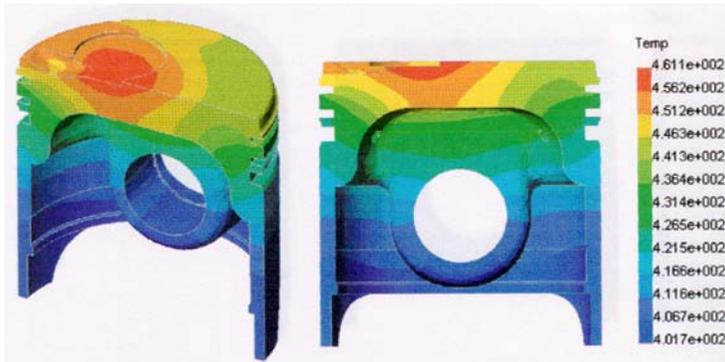
Fig. 6. Temperature (K) field in the composite piston for two different manufacturing of pistons
