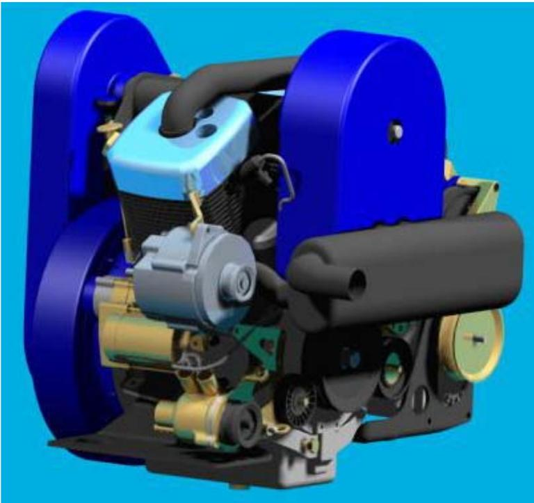
*Fig. 12. Compound Engine 999cc V Twin and conventional crankshaft*
