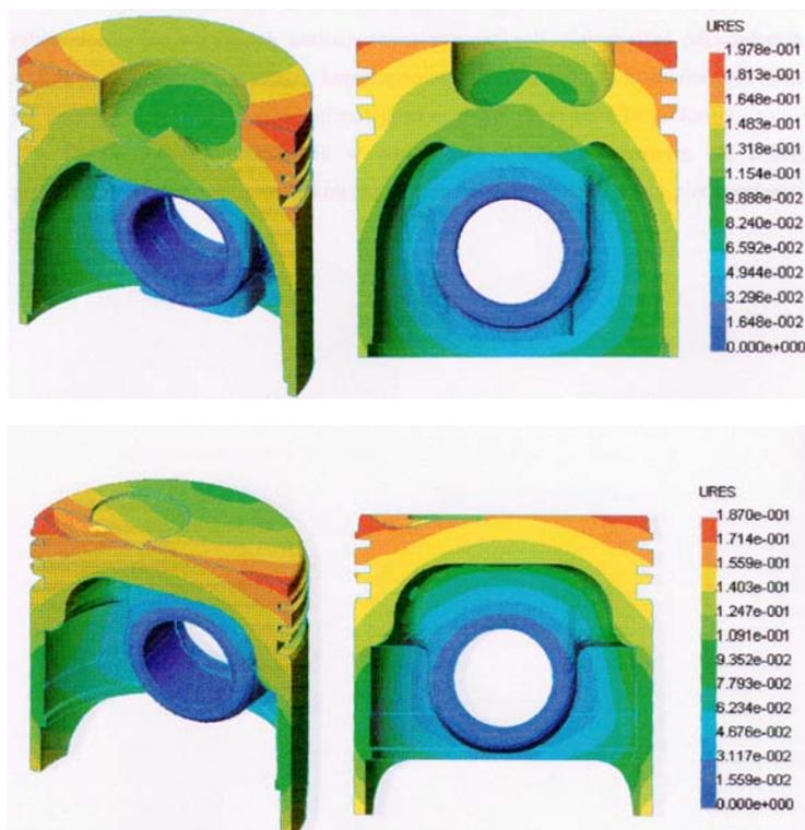
Fig. 8. Values of strains (mm) in the composite piston due to the temperature field for two different manufacturing of pistons
