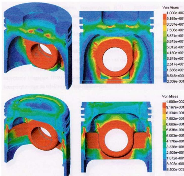
Fig. 7. Values of stresses (MPa) due to the temperature field in piston for two different manufacturing of pistons
